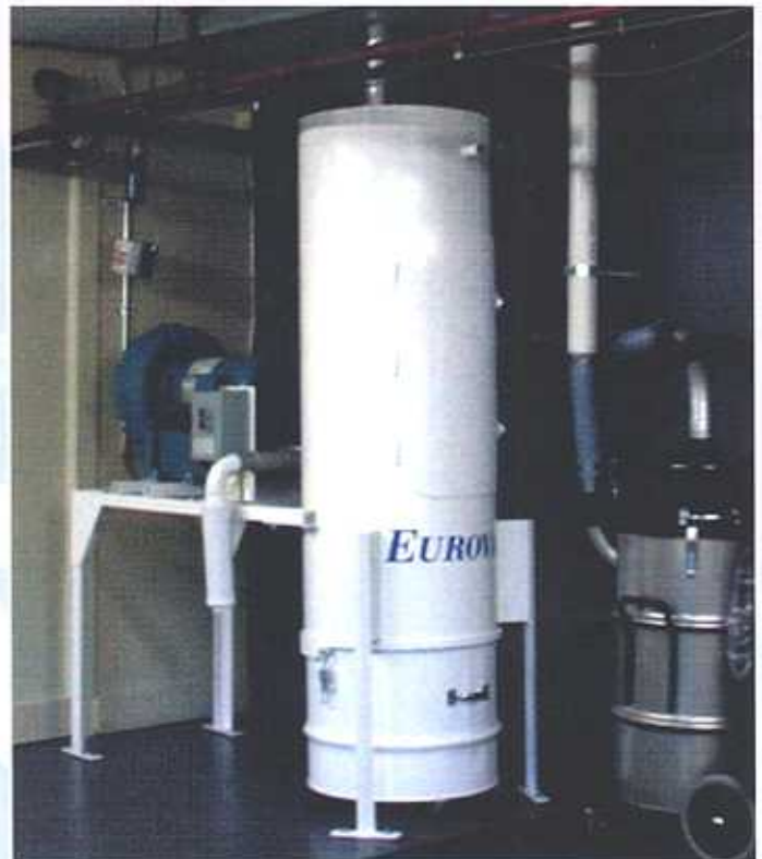
Eurovac I System with 7 HP or 10 HP Regenerative Blower and 10-bag Filter Separator
